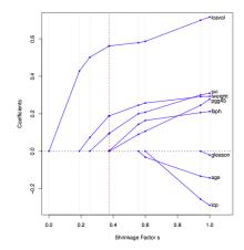
Shrinkage Factor  $s = r/|\hat{w}|_1$ , where  $\hat{w}$  is the ERM (the unpenalized fit).
