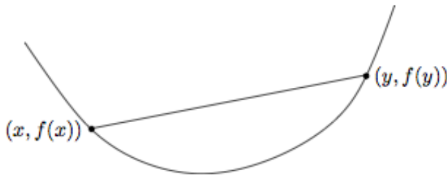
Figure 3.1 Graph of a convex function. The chord ( i.e. , line segment) between any two points on the graph lies above the graph.
